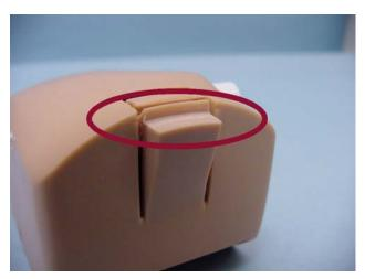
Battery latch height adjustment
